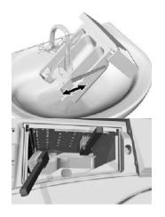
• Clean the entire rinsing area of the washing machine with a brush, especially the nozzles on the upper side of the rinsing chamber.
