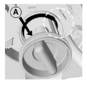
• Insert the filter back as shown on the picture (arrow and pointer), and tighten by turning it in clockwise direction. To ensure good sealing the gasket surface (A) must be dirt free.
